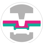
Clinching. TOX ® -Sheet Metal Joining
