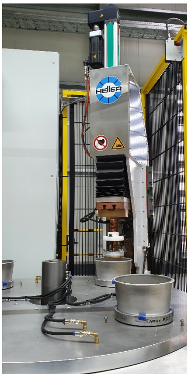
Image 4: The servo drive TOX-ElectricDrive individually adapts the stroke of the welding electrode to the respective pot size.
