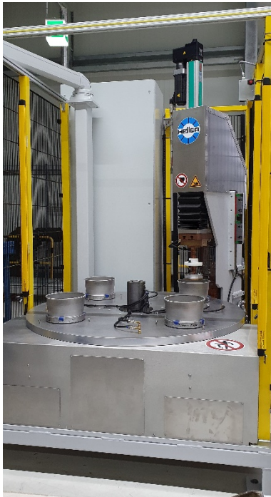
Image 1: While the machine bonds at the rear, the operator can newly equip the two front nests.
